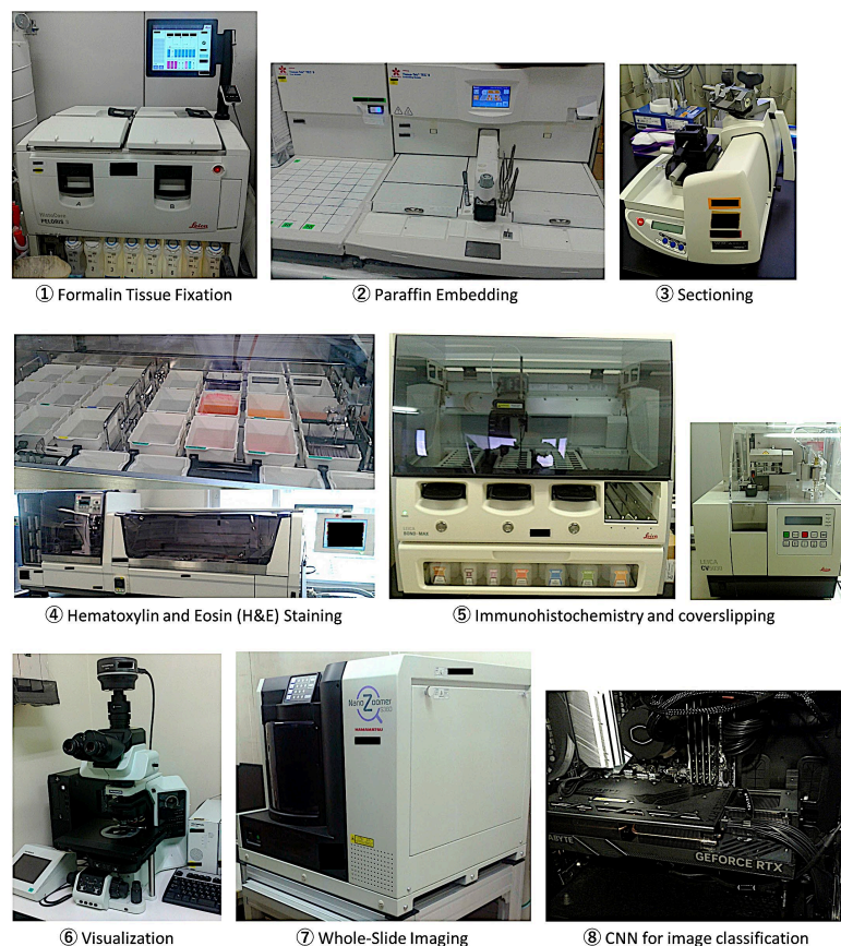
Figure 3. Workflow for Deep Learning Image Classification of histological images. This study analyzed and classified hematoxylin and eosin (H&E) histological images of follicular lymphoma and reactive lymphoid tissue (follicular hyperplasia). The steps of tissue fixation, paraffin embedding, sectioning, staining, visualization, digitalization, and CNN classification using an NVIDIA 4080 super graphic processing unit are shown in order. Of note, in the differential diagnosis between follicular lymphoma and reactive tissue, additional immunohistochemical stainings and molecular techniques could be required.
